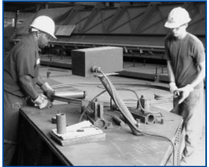
At the Tampa Fabricated Reinforcing Steel Division, Rebar Bender Johnny Harold, left, and Shipper, Checker, Loader Jon Erdly bend circular T-3s for the Reversible bridge segments.
