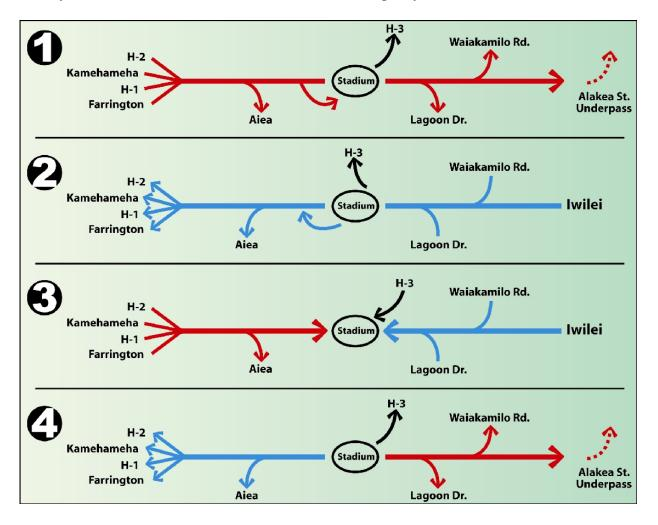
The HOT expressway can be configured to work in four different ways, depending on traffic loads and traffic management needs. The red direction is Koko Head-bound, and the blue direction is Ewa-bound.
